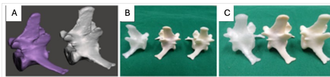
Figure 1 - (A) 3D reconstruction images of lumbar vertebrae L5 (left) and L4 (right) obtained from CT scans of the corresponding macerated vertebrae. (B) Photographic images of L4 vertebral models in PLA (left), macerated (center), and ABS (right). (C) Photographic images of L5 vertebral models in PLA (left), macerated (center), and ABS (right).
